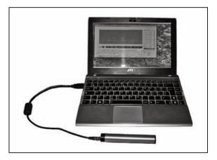
Figure 1. Ultrasound USB recording set: Asus Eee PC 1225B notebook personal computer, USB cable and Dodotronic Ultramic 250. On the display, SeaWave software by the University of Pavia's Interdisciplinary Center for Bioacoustics.
