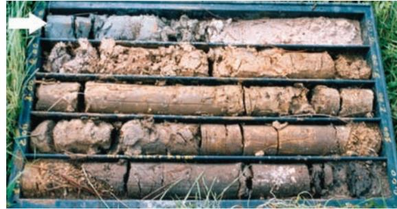
Fig. 2. Core photograph, showing the first 5 meters from ground level; the arrow indicates the portion of the borehole where it was found the Tyrrhenian malacofauna described
